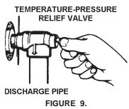
If after manually operating the valve, it fails to completely reset and continues to release water, immediately close the cold water inlet to the water heater, follow the draining instructions, and replace the temperature-pressure relief valve with a new one.
